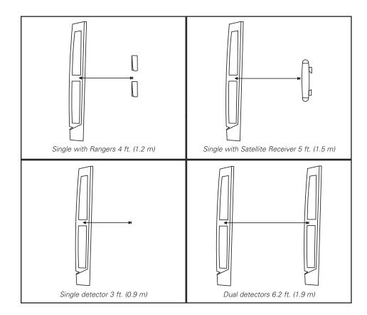
covers both with a choice of a single detector system for openings 3 ft. (0.9 m) wide or dual systems for opening 6.2 ft. (1.9 m) wide.
