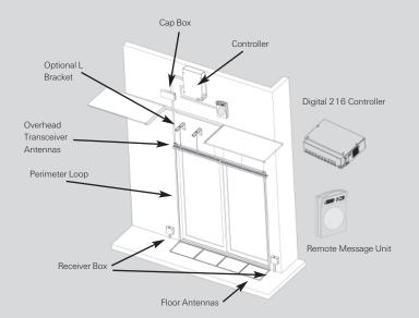
The Ultra-Loop 5 Meter System consists of a controller, transmit and receive antennas, two overhead transceiver antennas and an alarm or message unit. The transmitter perimeter loop is a cable that surrounds the doorframe. Two floor loops are used as receivers. The system operates with the ADS 216 Digital Controller.
